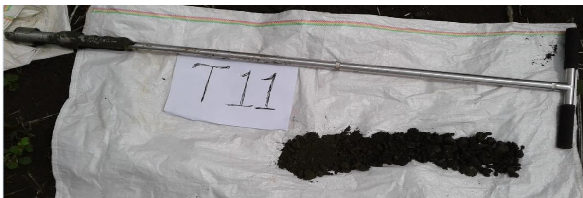
Figure 8-8: Photograph showing Bonheim / Luvisol soil profile – Tigray IAIP site
