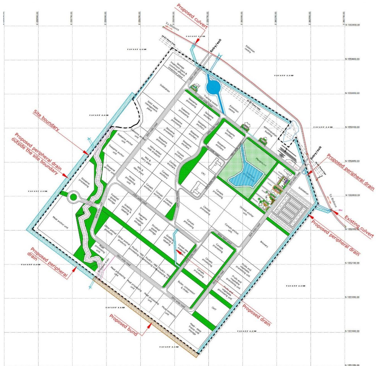
Figure 2-4: Site layout plan of the Baeker IAIP (Source: MACE Master Plan_MACE-P942-WT-BA-MP-001, dated 04/09/2017)
